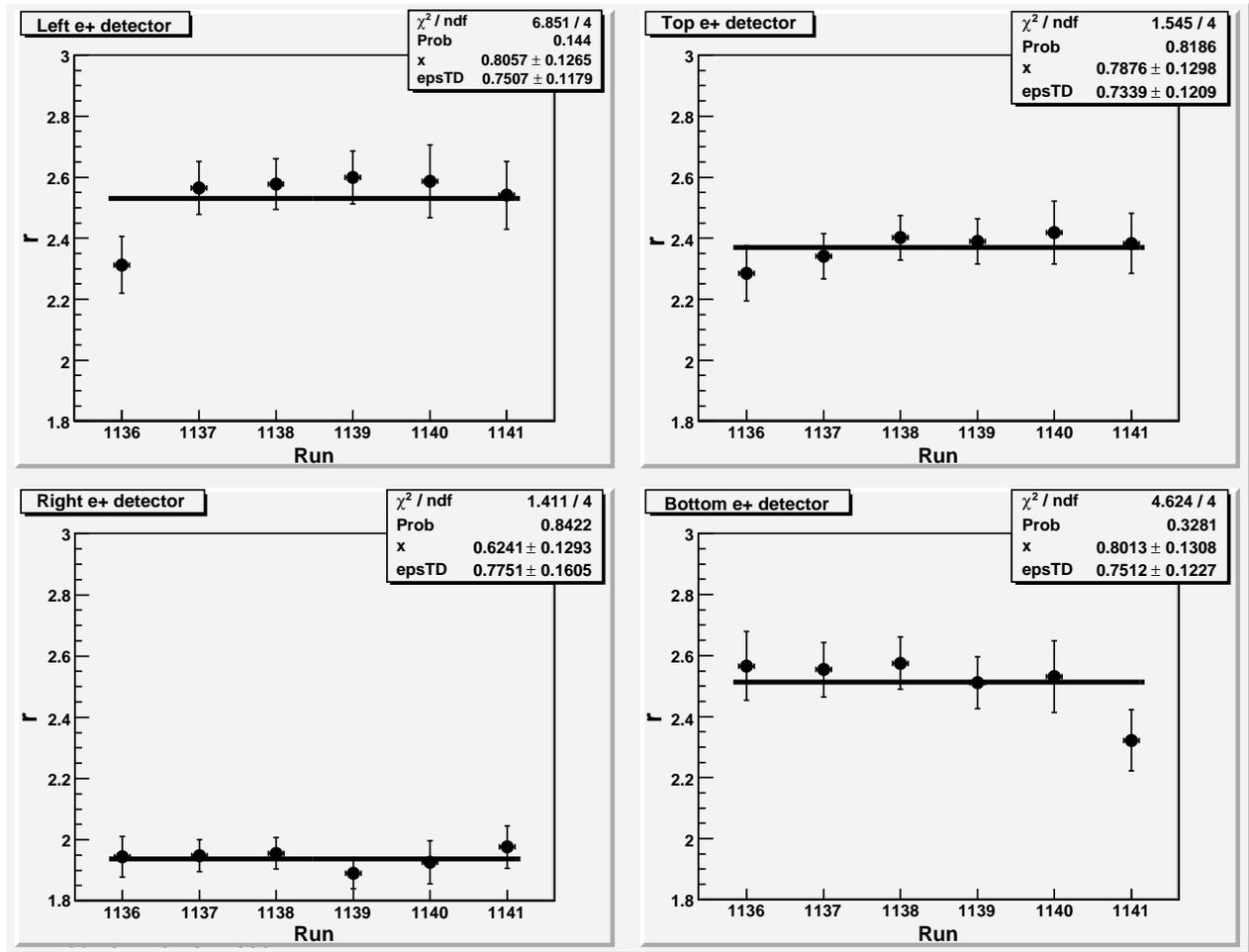
Figure 3: Fit of Eq. 5 to the data to determine  $\varepsilon_{TD}$ . Due to the strong correlation with the 2nd fit parameter  $x$  (which in principal could be fixed, because it can be determined experimentally) the errors of the fit are large. But this figure is just to demonstrate, how it works.
