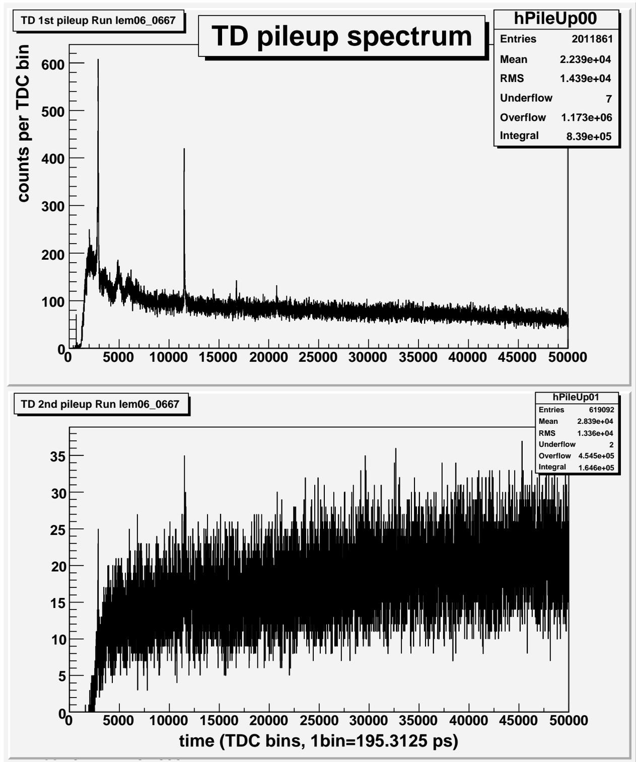
Figure 4: Measured post-pileup spectrum of the “trigger detector”  $TD$ . Shown are the spectra of the 1st and 2nd post-pileup hit. The peaks are partially *real*, i.e. they move when changing the transport energy of the LEM apparatus, and partially generated by the electronics.
