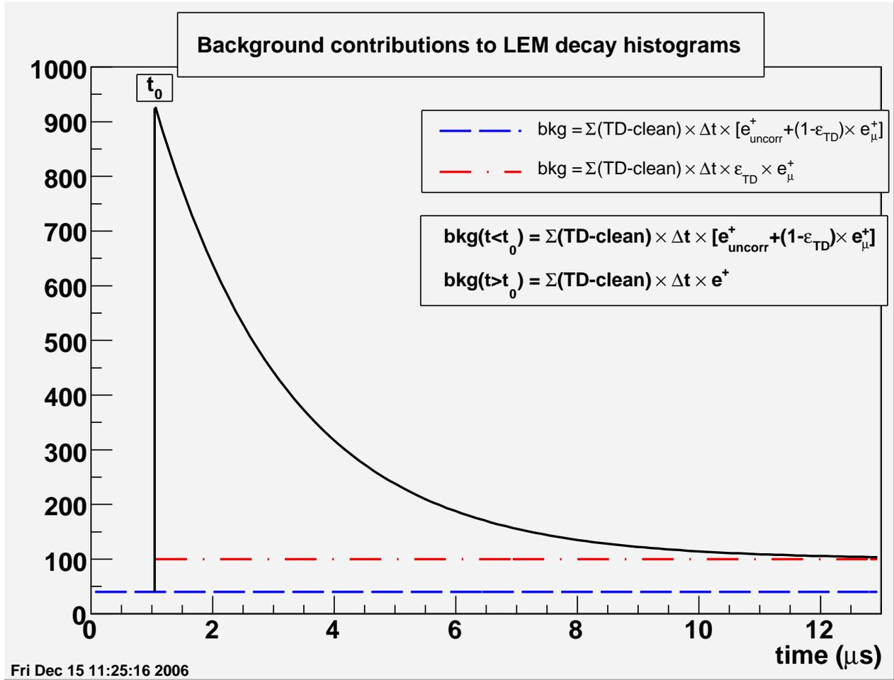
Figure 1: Background contributions to the LEM raw decay histograms. The difference in background between  $t < t_0$  and  $t > t_0$  arises from the non-rejection of post-pileups in the LEM data acquisition logic, as described in the text. Here,  $\Sigma(TD_{\text{clean}})$  is the total number of  $TD_{\text{clean}}$  in a run,  $\Delta t$  is the bin width,  $e^+ = e^+_{\text{uncorr}} + e^+_{\mu}$  is the measured positron rate, and  $\epsilon_{TD}$  is the detection efficiency of  $TD$ .
