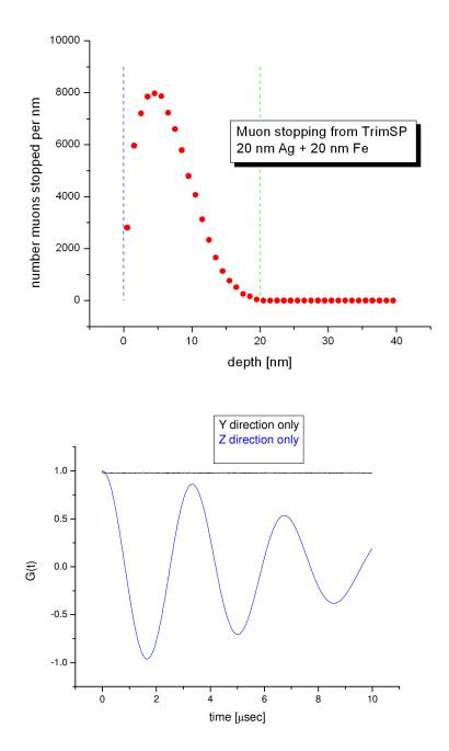
Note that the oscillation for the z-direction is due to the finite size of the sample.
