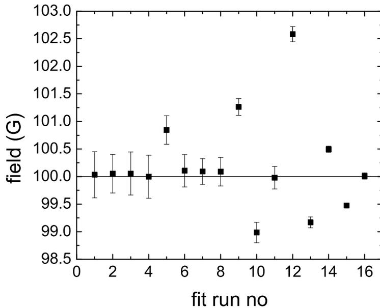
Figure 7: Fit results for the field  $B_0$  of the fake data test *with* TF background. The fit run no 1...8 correspond to a skewed Gaussian fit of the data set no 9...16 of Tab.1. The fit run no 9...16 are the results of a purely Gaussian (including the TF background) fit to the same data set.
