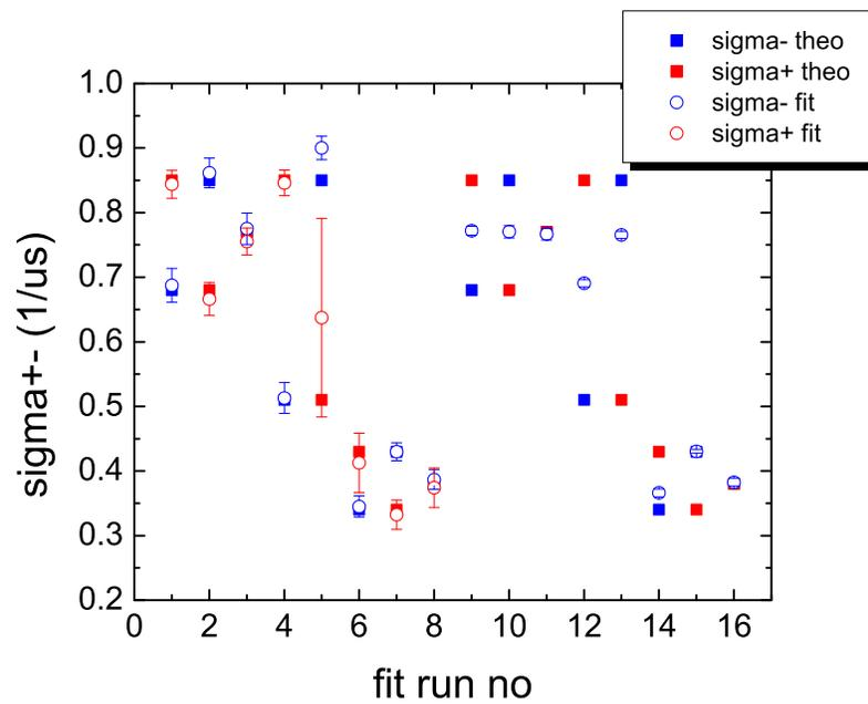
Figure 8: Fit results for  $\sigma_-/\sigma_+$  of the fake data test *with* TF background. The fit run no 1...8 correspond to a skewed Gaussian fit of the data set no 9...16 of Tab.1. The fit run no 9...16 are the results of a purely Gaussian fit (including the TF background) to the same data set. The open symbols are the fit results, whereas the full symbols show the theoretical values.
