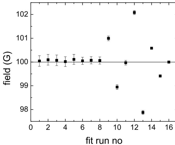
Figure 5: Fit results for the field  $B_0$  of the fake data test *without* TF background. The fit run no 1...8 correspond to a skewed Gaussian fit of the data set no 1...8 of Tab.1. The fit run no 9...16 are the results of a purely Gaussian fit to the same data set.
