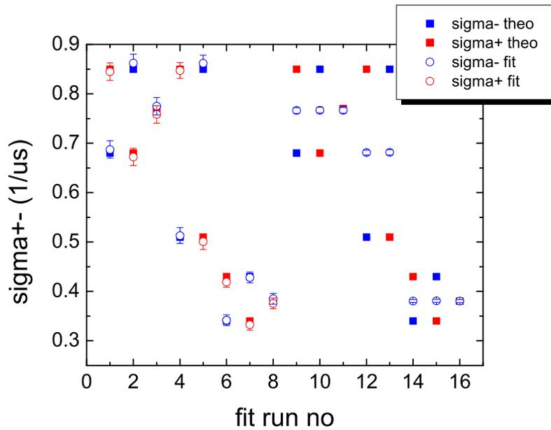
Figure 6: Fit results for  $\sigma_-/\sigma_+$  of the fake data test *without* TF background. The fit run no 1...8 correspond to a skewed Gaussian fit of the data set no 1...8 of Tab.1. The fit run no 9...16 are the results of a purely Gaussian fit to the same data set. The open symbols are the fit results, whereas the full symbols show the theoretical values.
