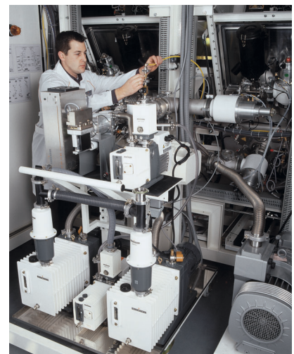
Pumping unit integrated in an industrial Leak Detection Systems
