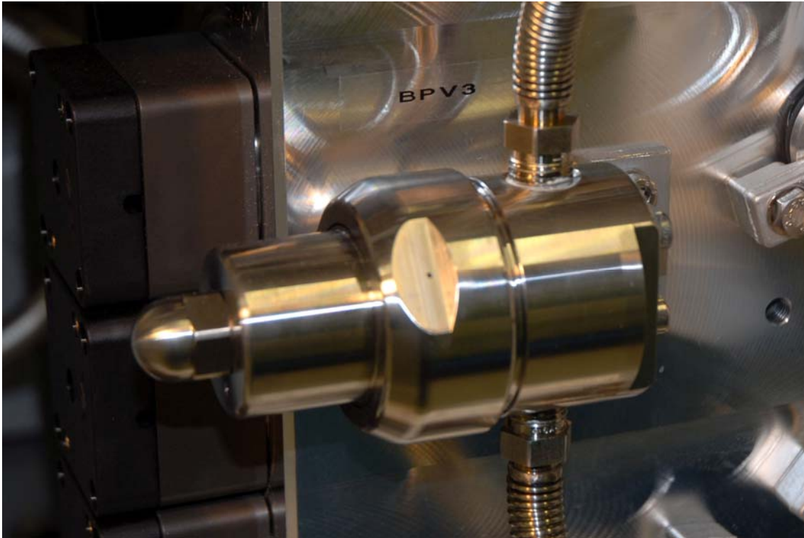
Figure 22. Backing pressure valve BPV3.
