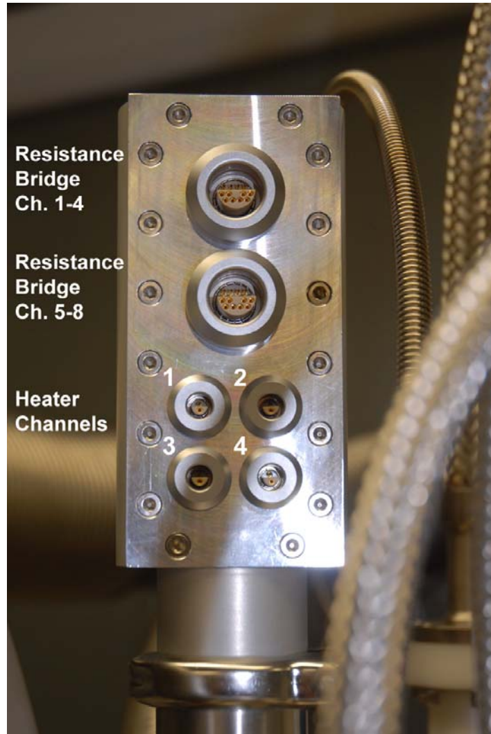
Figure 15. DR wiring connector box.
