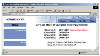
**embedded web server** allows the instrument to be viewed and configured from any web browser. An example 'Status' page is shown here.
