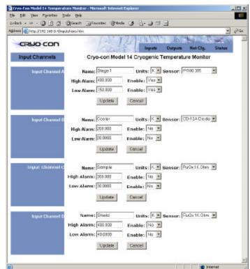
**Software:** Utility software is provided that connects any Windows based personal computer to either monitor. This software provides a graphical control panel that greatly simplifies instrument setup and configuration.
