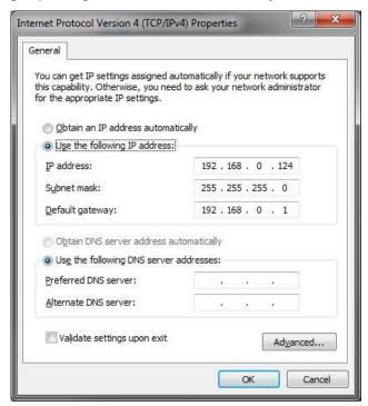
2.3.6. The DNS server settings can be left blank. Hit **Ok** to return to the **Local Area Connection Properties** window and then hit **Ok**. **Local Area Connection** should show that it is connected. If it is not able to connect, double check the IP address settings for both the LM-510 and the ethernet adapter.
