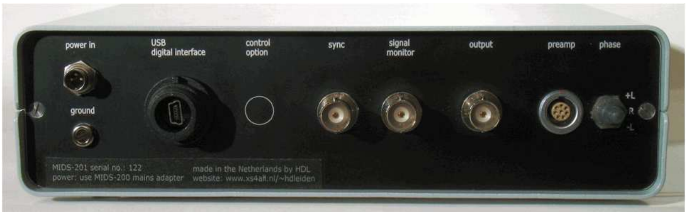
MIDS-201 1-channel control unit, back side
