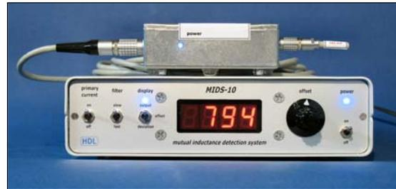
**Figure 2.13.** The test plug connected to the preamplifier; the control unit displays the value as indicated on the plug.
