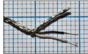
Figure 2.4. Cryogenic shielded twisted pair cable.
