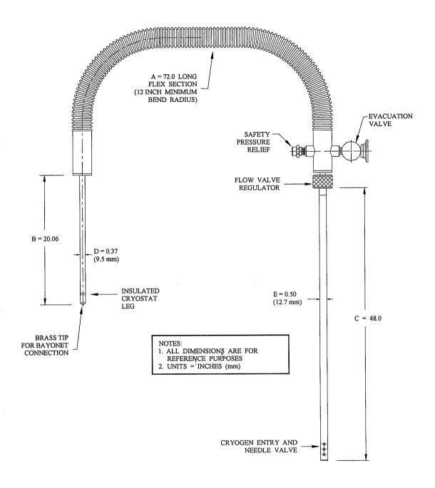
Figure 1: Model FHT-ST high efficiency flexible helium transfer line
