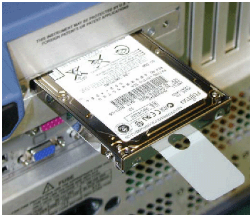
Proper Orientation of Drive
