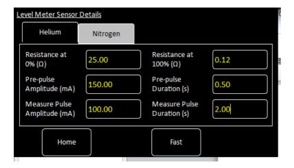
Figure 16-3 Level Meter Sensor Details page - Helium tab
