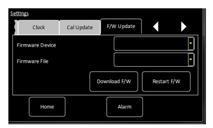
The page allows the user to update the firmware on a daughter board. The new firmware must be located on a USB memory stick. The page contains the following fields and controls:
