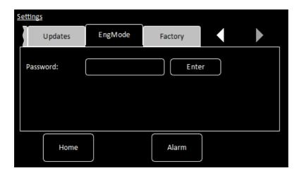
This page allows the user to enter *ENGINEERING* mode, to access features that are not available to normal users. The default engineering password is **abc123**. The user can change this password, if required.
