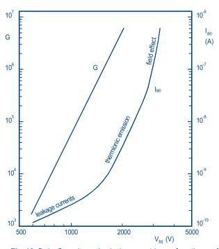
**Fig.13** Gain G and anode dark current  $I_{a0}$  as functions of the PMT supply voltage, showing the voltage regions in which each of the three main causes of dark current predominates.
