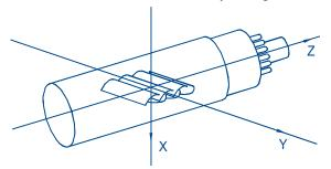
Fig.37 Axes used in measuring magnetic sensitivity.
