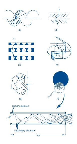
**Fig.8** Dynode configurations of electron multipliers: (a) linear focusing, (b) venetian blind, (c) foil, (d) box, (e) circular cage and (f) MCP.
