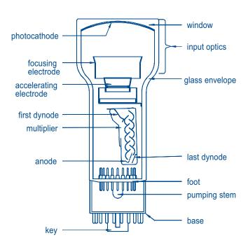
**Fig.1:** Main elements of a photomultiplier. (Based on the fast 3" basic tube, the XP4312B).
