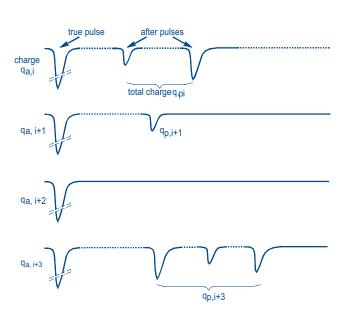
**Fig.16** Examples of the development in number and charge of afterpulses.  $q_{a,i}$  etc. is charge transferred by true pulses;  $q_{b,i}$  etc. that transferred by afterpulses.
