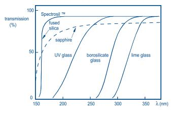
Fig.3 Transmission as a function of wavelength  $\lambda$  for various glasses used in photomultiplier input windows.
