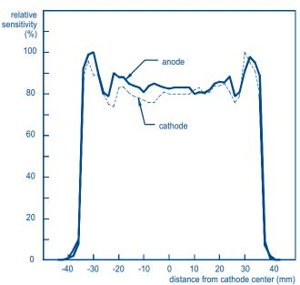
**Fig.5** Example of anode and cathode sensitivity variation measured at  $\lambda$  = 424 nm along one diagonal of a XP3692, 60 mm square PMT with SbKCs cathode.
