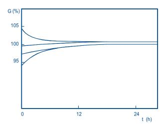
Fig.25 Examples of initial low-current drift.
