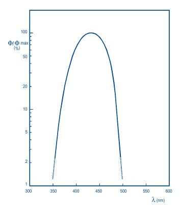
**Fig.4** Relative spectral characteristic of 2856 K tungsten light transmitted by a Corning CS 5-58 filter ground to half stock thickness.
