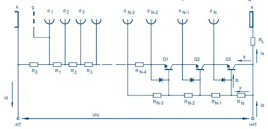
Fig.31 Using transistors to keep constant inter-electrode voltages on the last stages, even at high count rates.
