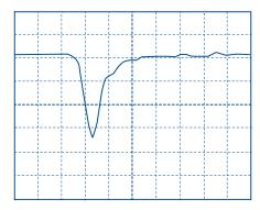
**Fig.20** Anode pulse response of a fast-response PMT. Vertical scale, 100 mV/div Horizontal scale, 5 ns/div.
