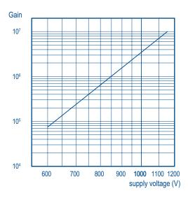
Fig.11 Published gain curve for XP2042 tubes.
