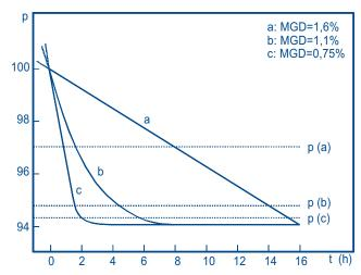
**Fig.26** Anode sensitivity curves showing the same absolute change over 16 hours but different values of mean gain deviation (MGD) according to the ANSI method (p(a), p(b) and p(c) are the corresponding mean heights of the pulse peak average over 17 readings).
