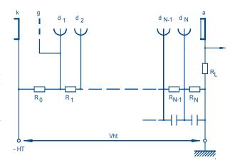
Fig.29 Negative-polarity voltage supply.
