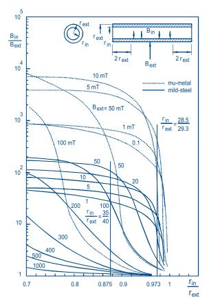
**Fig.38** Comparative effectiveness of mu-metal and soft iron magnetic shields.
