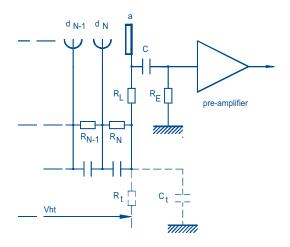
**Fig.30** Network for decupling the high-voltage switch-on transient from the amplifier input.
