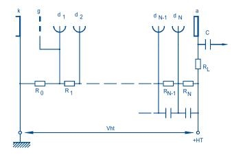
Fig.28 Positive-polarity voltage supply.
