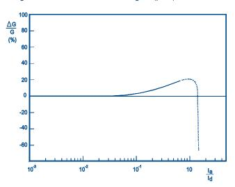
Fig.22 Gain variation (overlinearity) as a function of the ratio I<sub>a</sub>/I<sub>d</sub>
