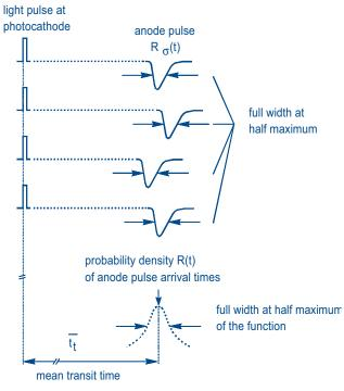
**Fig.21** Response-pulse jitter due to transit-time fluctuations.
