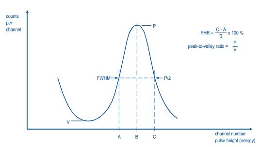
Fig.17 Typical pulse height spectrum showing the definition of pulse height resolution and peak-to-valley ratio.
