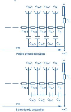
Fig.32 Parallel and series dynode decoupling.
