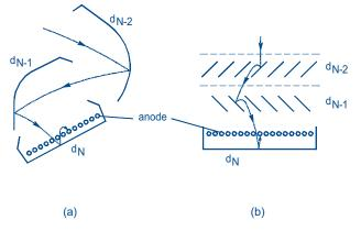
**Fig.12** Collection-space configurations: (a) with focusing dynode, (b) with venetian-blind dynodes.
