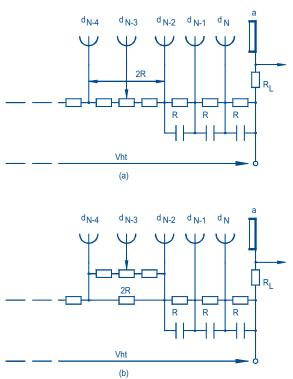
**Fig.34** Alternative circuits for adjusting gain by adjusting the voltage of one dynode.
