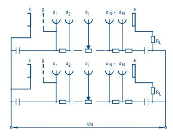
Fig.36 High voltage supply for photomultipliers in parallel.
