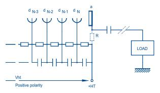
**Fig.33** Fixing the anode potential with the tube connected in negative or positive polarity.
