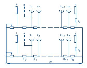
Fig.35 High-voltage supply for photomultipliers in parallel.
