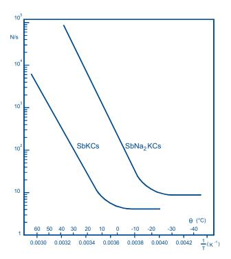
**Fig.14** Number of dark pulses per second as a function of temperature for SbKCs and SbNa<sub>x</sub>KCs photocathodes.
