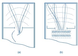
**Fig.7** Input electron-optics of a PMT with (a) focusing dynodes and (b) venetian-blind dynodes, showing equipotential lines and electron trajectories.
