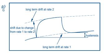
Fig.27 Long-term gain drift and short-term shift due to change of operating conditions.
