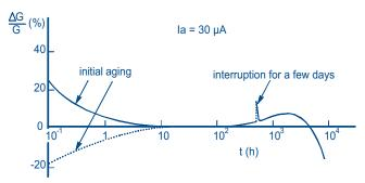
**Fig.24** Relative gain variation of a PMT operating at high average current.
