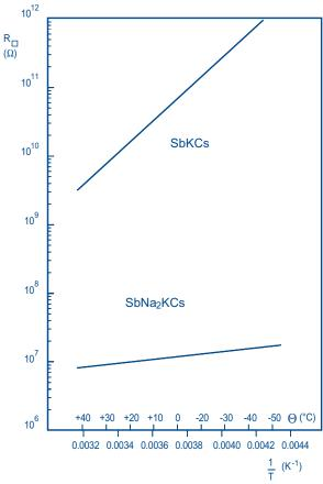
**Fig.40** Surface resistivities of two photoemissive materials as functions of temperature.
