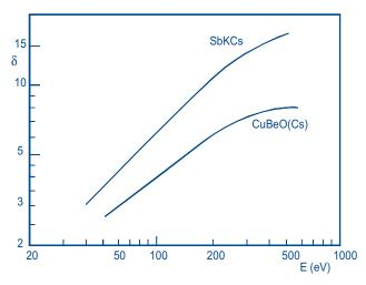
**Fig.9** Secondary emission coefficients,  $\delta$ , of the commonly used dynode materials, as functions of incident primary-electron energy, E.
