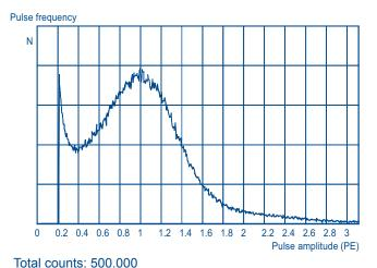
**Fig.15** Example of dark-current spectrum with linear focused dynodes. (XP2960 tube).
