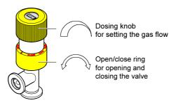
Rotating the dosing knob translates into a linear movement and places the dosing needle reproducibly in the desired position.
