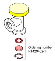
Filter vacuum side (gas flow 1250 mbar l/s)
