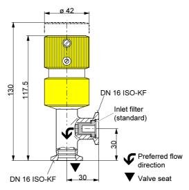
Gas flow with standard filter 1700 mbar I/s Gas flow without standard filter 3100 mbar I/s
