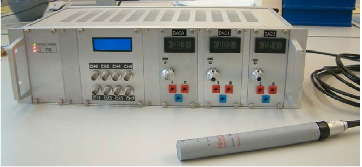
Figure 2: Zero-field compensation control unit together with the 3-axis fluxgate probe.
