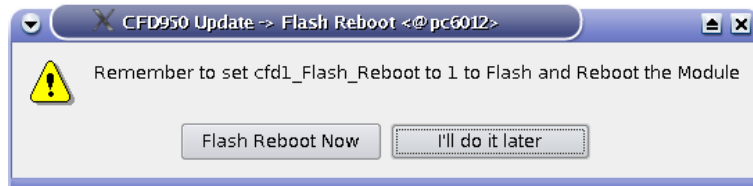
Figure 10: Dialog to perform a flash & reboot of the CFD.
