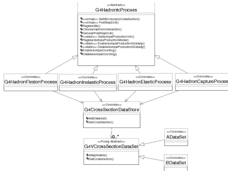
Figure 3.2. Level 2 implementation framework of the hadronic category of Geant4; cross-section aspect.
