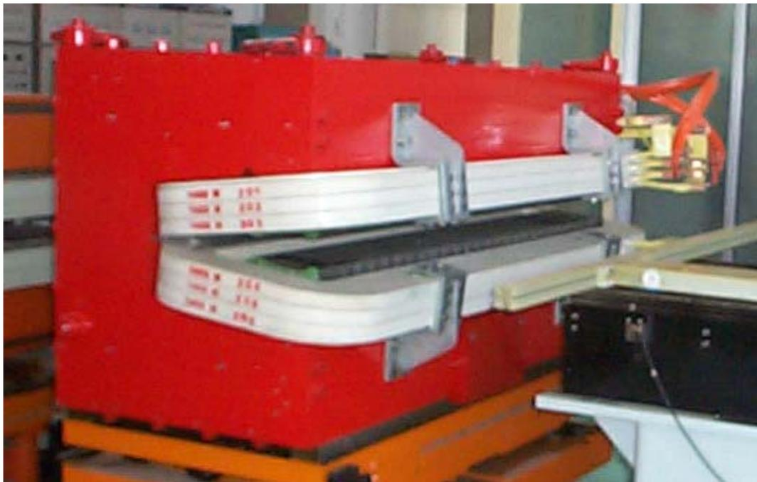
Figure 2 SPEAR3 Gradient Dipole Magnet
