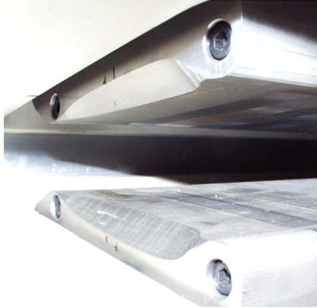
Figure 4 Chamfer on Prototype Gradient Magnet Removeable Pole Ends
