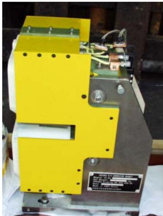
Figure 6 SPEAR3 Combined Horizontal and Vertical Steering Corrector
