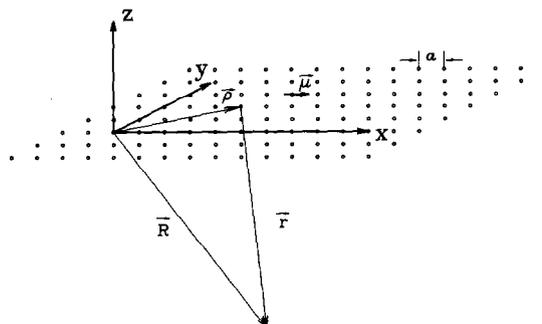
Fig. 1. Plane square lattice of magnetic moments.  $\mathbf{R}$  denotes the radius-vector of a point where the dipolar field is calculated.
