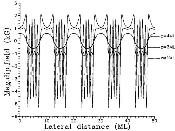
Fig. 3. Calculated profile of the magnetic dipolar field, created by the imperfect layer (Fig. 2) at various distances  $z$  for bcc-structure of iron and  $L = 10$  ML.
