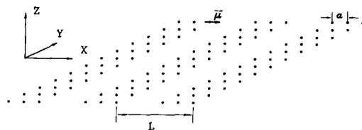
Fig. 2. Imperfect layer corresponding to a rough surface consisting of an array of infinitely long monoatomic terraces and valleys with period  $L$  and width  $L/2$ . The magnetization is supposed to be aligned in  $x$ -direction.
