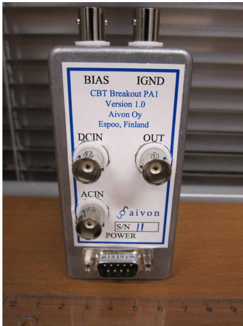
Figure 1: CBT current preamplifier PA1
