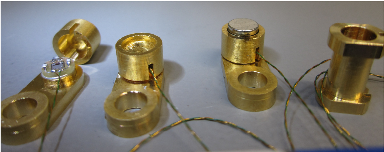
Figure 1: The sensor H3L3 consists of two gold-plated copper parts, lid and holder. From left to right: Opened sensor, sensor H3L3, sensor H3L3m with magnet, and bobbin B1. The sensor wire is 30-cm long phosphor bronze twisted pair.
