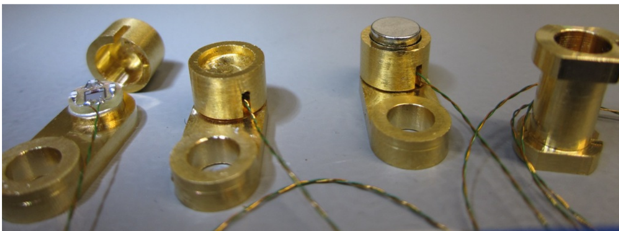
Figure 2: From left to right: Uncovered CBT sensor (holder/lid type H3L3), H3L3 as normally delivered, strong permanent magnet is glued on top of the lid (H3L3m), and bobbin B1 for thermal anchoring of the wire.
