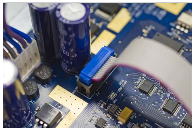
FIGURE 7-5 Proper orientation of the ribbon cable connector plug
