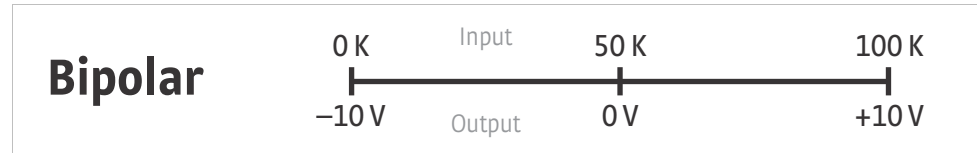
FIGURE 5-3 Analog output with polarity set to bipolar
