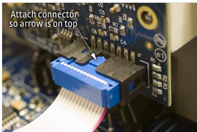
FIGURE 7-5 Proper orientation of the ribbon cable connector plug
