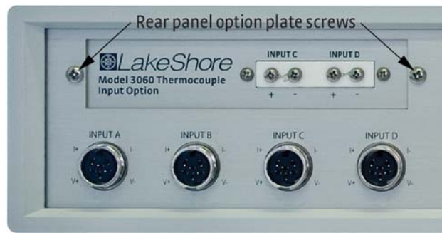
FIGURE 7-4 Align the 3060 card with input C and D
