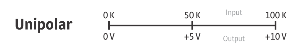
FIGURE 5-4 Output with polarity parameter set to unipolar
