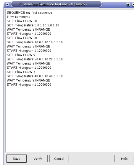
Figure 2.14: Editor window containing the file to be edited. Once the editing is finished, the user has the possibility to verify the autorun syntax, and save the file.
