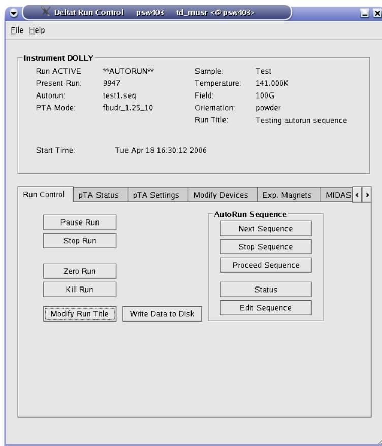
Figure 2.23: Main window indicating that an autorun sequence is active (note the **AUTORUN** indication at the top of the window). Note also that the interactive button (as Stop Run , etc...) are in the autorun mode only active when a run is active.
