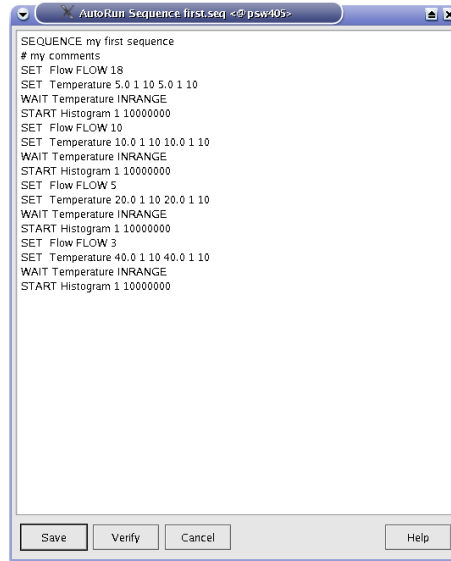
Figure 2.22: Editor window containing the file to be edited. Once the editing is finished, the user has the possibility to verify the autorun syntax, and save the file.
