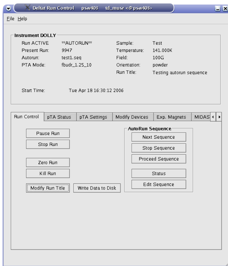
Figure 2.32: Main window indicating that an autorun sequence is active (note the **AUTORUN** indication at the top of the window). Note also that the interactive button (as Stop Run , etc...) are in the autorun mode only active when a run is active.
