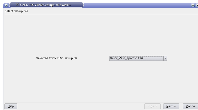
Figure 2.26: The first wizard tab will prompt you for the name of the TDC-setting file.
