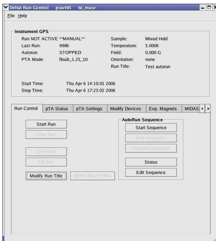
Figure 2.1: deltat main window with the Run Control tab selected. Note that a run is not active and that the mode is manual. Note also that the Start Run button is clickable.
