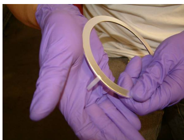
Figure 3.7: Preparing a new 100CF copper gasket with sticky tape.
