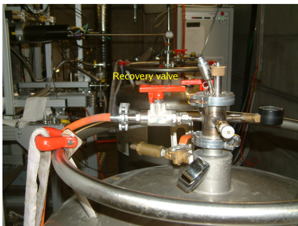
Figure 6.1: Red Recovery-line-valve on the He dewar
