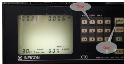
Figure 4.8: The XTC unit for measuring the thickness of moderator layers
