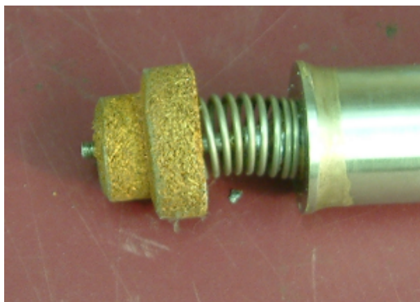
Figure 7.28: LowTemp-2 cooler, lowest part with sinter for maximal thermal contact
