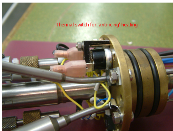
Figure 7.25: Thermal switch for anti-icing heater.
