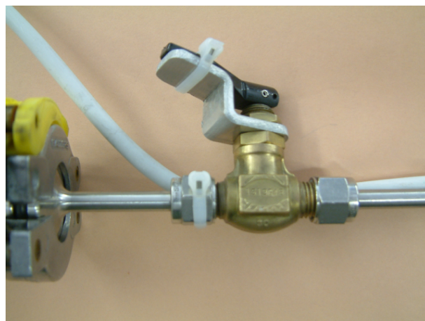
Figure 7.39: Correct way of closing the vacuum valve, including security wrap
