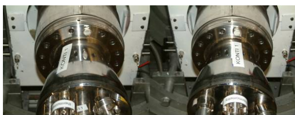
Figure 3.8: Konti-1 positioned incorrectly (left) and correctly (right). The exact orientation does not affect the operation of Konti cryostats.
