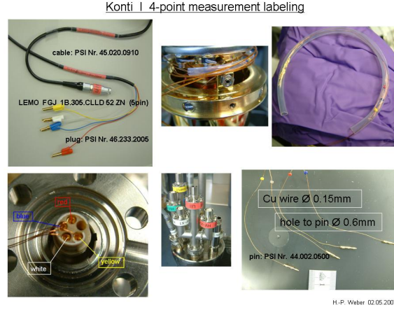
Figure 7.9: Connection for the 4-point resistance measurement.
